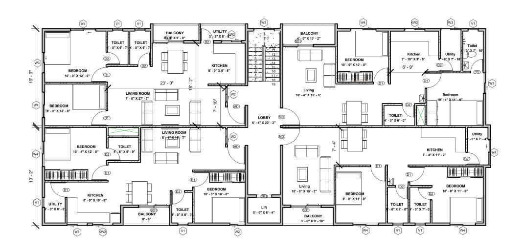
WALL THICKNESS: EXTERNAL WALL=6" INTERNAL WALL=4"
