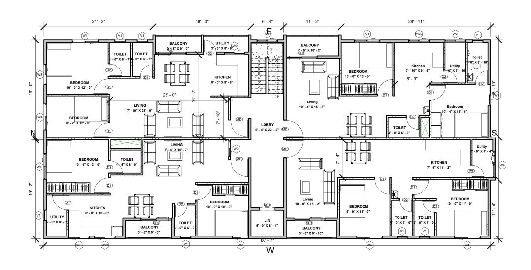
WALL THICKNESS: EXTERNAL WALL=6" INTERNAL WALL=4"
