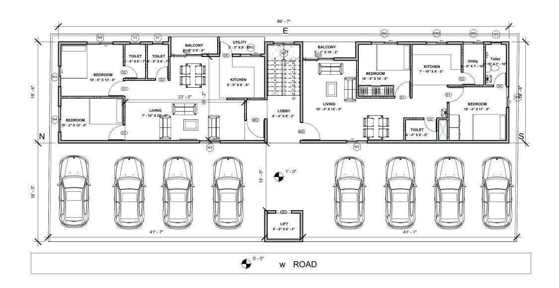
**WALL THICKNESS: EXTERNAL WALL=6"** INTERNAL WALL=4"
